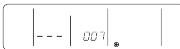
LOSSNAY can be searched in the same manner by bringing up the LOSSNAY address in the Interlocked unit address display window.
